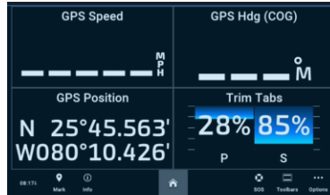
Displays trim tab positions on multifunction display
